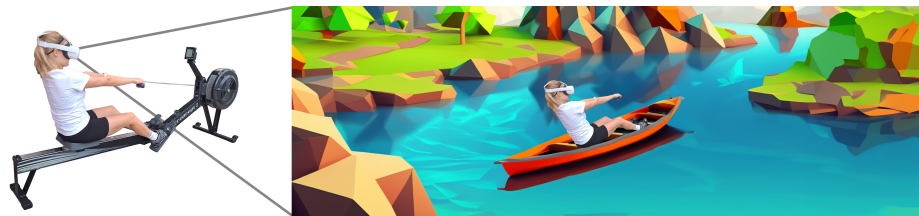
Figure 1: VRow allows for easy integration of ergometers, like the rower in this example, into Virtual Reality applications for synchronous fitness training.
