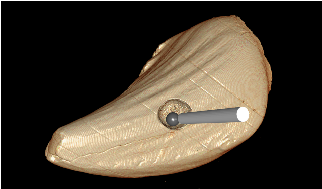
Figure 1: Sculpting of an Ornithischian tooth. As a user activates the sculpting function and the virtual probe collides with the tomographic volume, affected voxels are removed.
