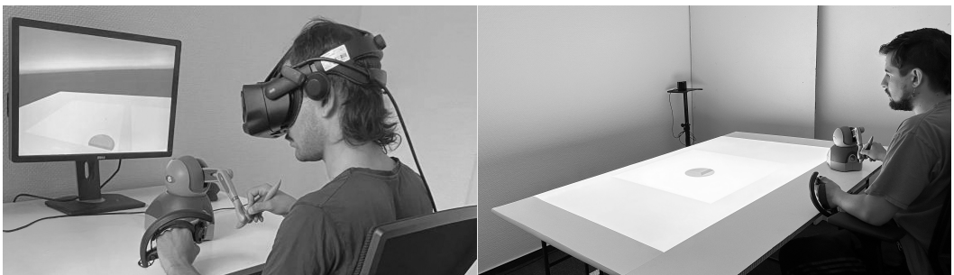
Figure 2. Left: a participant in our original VR study [130] exploring a stimulus using an HMD and a grounded force-feedback device. Right: a participant in our projected surface study performing the same task while facing the stimulus on a projected surface.
