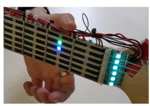
(a) LED: LEDs indicate which strings should be pressed.
