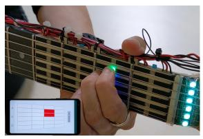
(c) LED-CS: Combination of LEDs and capacitive sensing.
