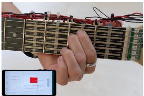
(b) CS: The touched fret is captured by capacitive sensing and visualized.
