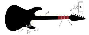
Figure 2: Schematic of *Let's Frets*. A Raspberry Pi (1) communicates via Bluetooth (2) with a smartphone app (6). The conductive frets (4) and LEDs (5) are connected via cables to the Raspberry Pi.
