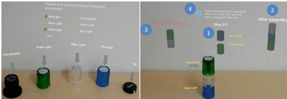
**Fig. 8.3** Lenssembly checks the available parts prior the assembly. **Left:** A checklist is displayed and an arrow with a description denotes the part. The assembly begins when all parts are available. **Right:** Lenssembly displays (1) the current procedure step, (2) the pre-trained result, (3) potential wrong actions, and (4) textual information messages that support the assembly
