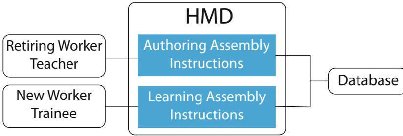
**Fig. 8.1** Application structure of Lenssembly. An Authoring Mode enables to create and author new assembly instruction procedures. The learning procedure uses the recorded instructions to transfer this knowledge to new workers via AR. A Playback Mode displays the assembly instructions in AR and verifies if the assembly is conducted correctly
