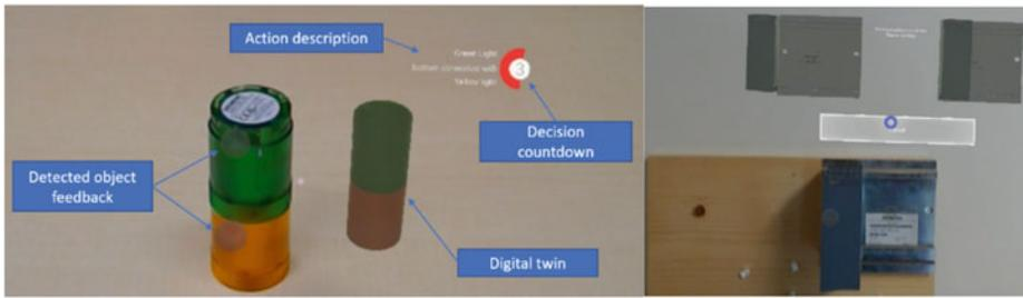
**Fig. 8.2** Procedure step suggestion process for a detected connected object in the Authoring Mode. **Left:** A connection between the yellow and green object was detected and is added to the assembly procedure after the decision timer expires. **Right:** Conflict resolution menu models two detected actions for the same objects. The user must choose one of the two actions by clicking on the corresponding model
