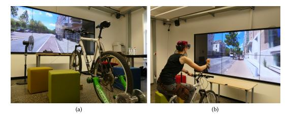
Fig. 2. Used setup for the study. (a): We used a bike simulator to imitate a realistic cycling scenario. The scenario itself is visualized on a video wall consisting of six screens. (b): A participant is interacting with gestures while using the bike simulator.
