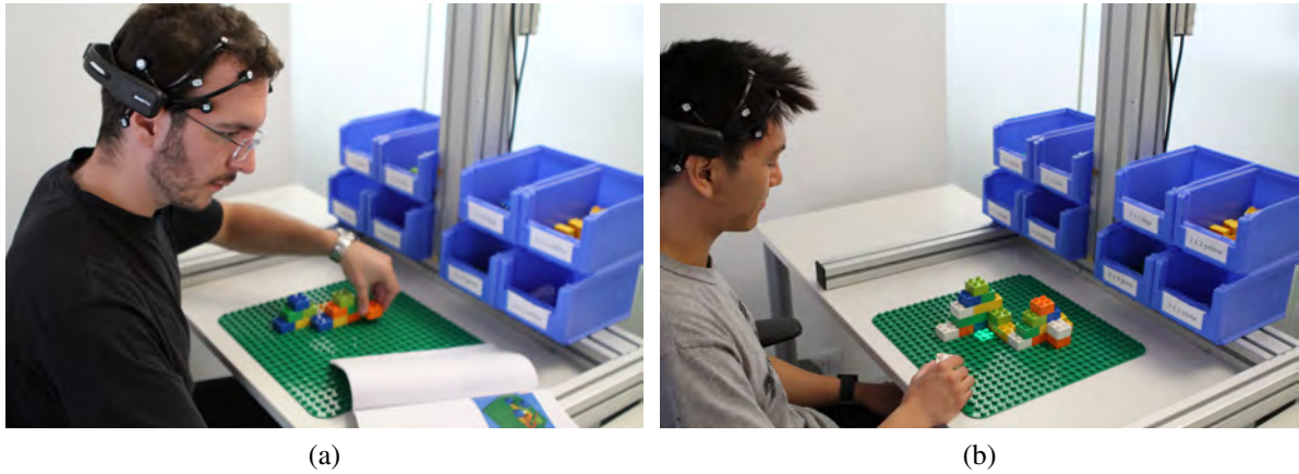
Figure 5.1: (a) Paper-based and (b) projected in-situ instructions at a manual assembly workplace. An EEG headset measures the level of working memory. This provides objective insights about the working memory load that is placed during manual assembly.
