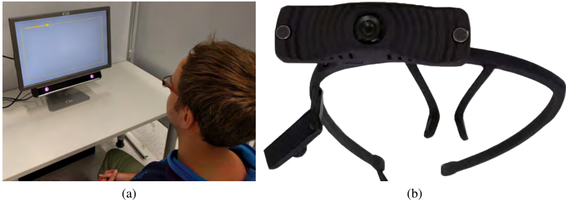
Figure 2.4: (a): Stationary eye tracker which emits infrared light. This light reflects on the cornea which is captured by the device to estimate the gaze points. (b): Head-worn mobile eye tracker. An infrared camera captures the reflection of infrared light and maps the gaze to a world camera.
