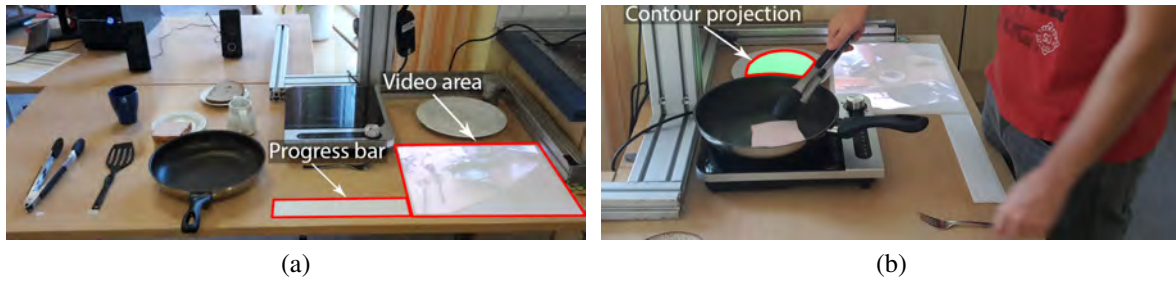
Figure 8.2: Visual output modalities of the cooking instruction system. (a): In-situ projections of video instructions and progress bars were displayed inside the cooking area. The projections were placed on white sheets to enhance the visibility. (b): In-situ projection of video instructions and contours which provide visual cues for grasping or placing objects and food.
