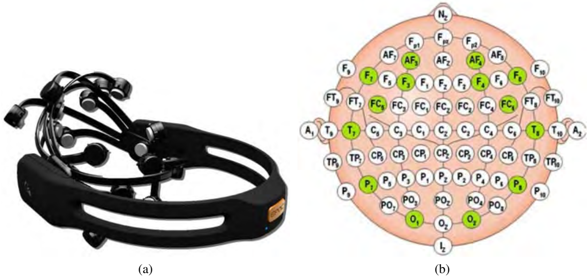
Figure 5.3: (a): The Emotiv Epoc wireless EEG headset featuring 16 electrodes including two reference electrodes. (b): Electrode placement layout of the 14 measurement electrodes [386].
