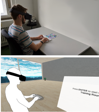
Figure 2: Top: User typing with our mixed reality apparatus. Bottom: The mixed reality environment with keyboard video texture and large floating display.
