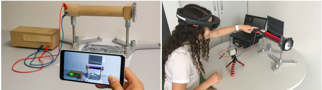
Figure 1: A person uses our prototype to understand thermal flux in a physics lab experiment. Users can either use a smartphone (left) or HMD (right) to extend their sight by thermal vision. Virtual elements are an extension for non-functional setups to simulate a real experiment.
