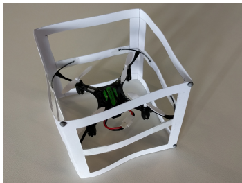
Figure 3: Quadcopter equipped with a cage to enhance tangible interaction.
