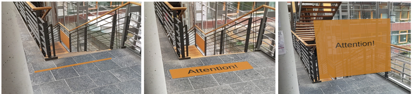
Figure 1: Mixed Reality devices could potentially warn its users about fall hazards such as staircases. In our explorative prototype study, participants tested three different warning types: A superimposed small line at the stair landing (Left), a bigger warning including a text label (Middle), and a full-scale warning blocking the whole stair entrance including a text label (Right).
