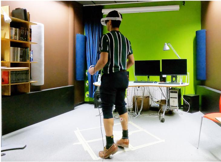
Fig. 11. Apparatus for Study II showing participant wearing the VR headset and attached electrodes on the calf.
