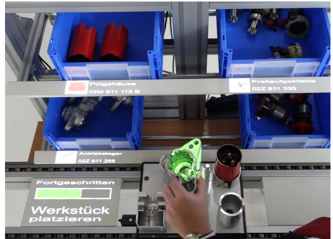
Figure 1. Our system assistive system for the manual assembly workplace uses in-situ projection to provide assembly instructions and uses motion recognition to become context-aware.
