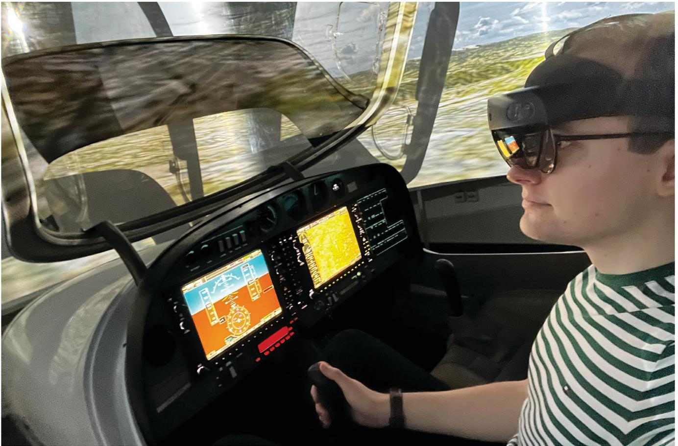
A pilot testing interaction with augmented en-route flight information through a mixed-reality headset in a high-fidelity Diamond DA40 simulator.
