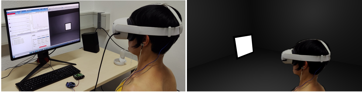
Figure 2: For our study apparatus, we use an Oculus Quest 2 VR-HMD and OpenBCI Ganglion EEG board. Left: A participant wearing a VR-HMD focused a stimulus. Right: The same participant in VR focusing on a black and white flickering square.
