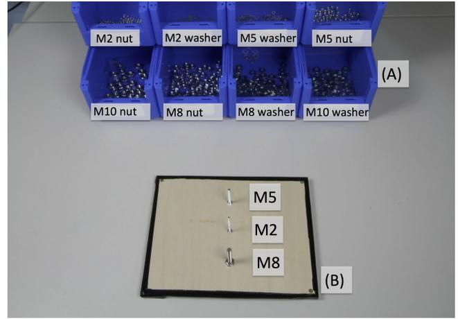
Figure 3. The apparatus of the assembly task. The assembly parts are stored in blue picking bins (A), the workpiece carrier (B) is placed in front of the boxes. The screws are aligned vertically that the worker can use both hands to for assembling the nuts and washers.
