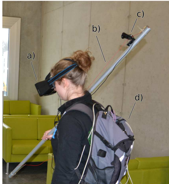
Figure 1: A user wearing our prototype. a) head-mounted display, b) camera stick, c) camera, d) backpack
