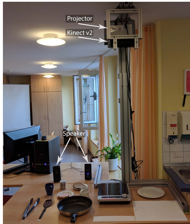
Figure 2: Study setup with pre-portioned ingredients. Auditory feedback is provided via external speakers while visual feedback is delivered by projections.
