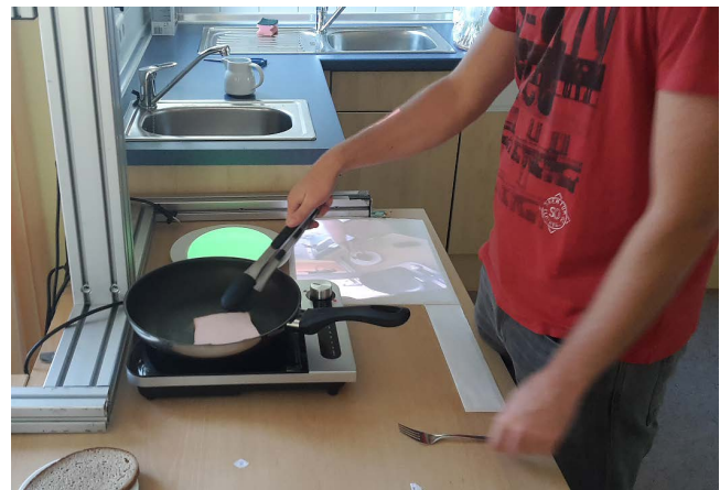
Figure 1: Assistive system providing visual and auditory in-situ assistance that supports people with cognitive deficiencies during cooking tasks.
