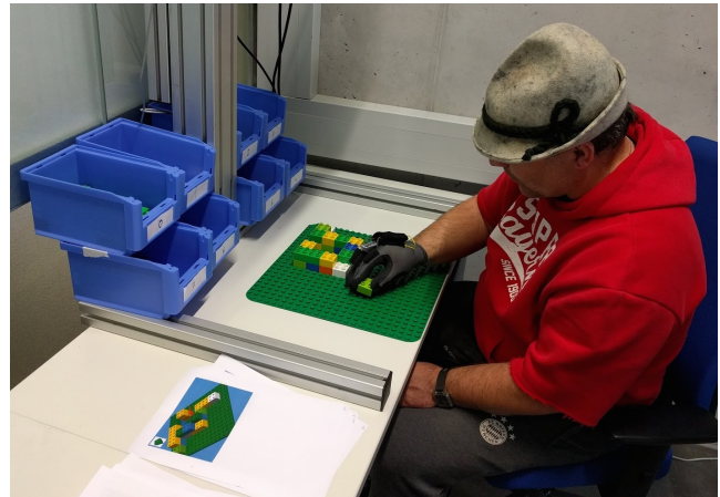
Figure 1: A participant is wearing an augmented glove providing tactile error feedback during assembly tasks.
