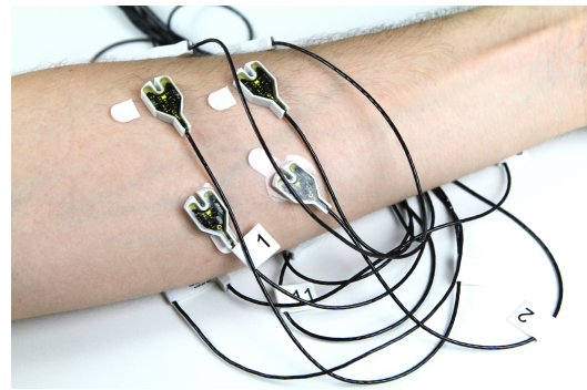
Figure 2. Electrode configuration with two rings around the forearm each consisting of five electrodes.
