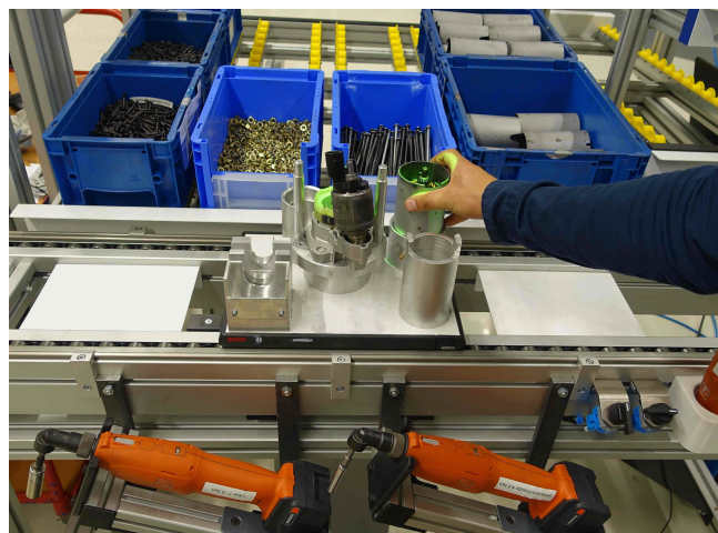
Figure 1. A user is working on an interactive workplace. A projector is displaying in-situ instructions directly on the work piece while a Kinect.v2 checks for correct assembly.
